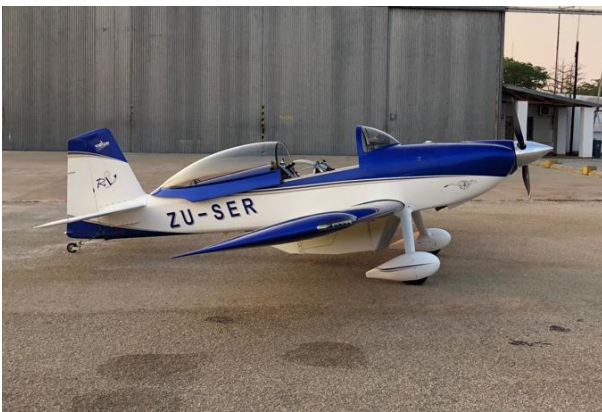
Figure 6: RV8 aircraft equipped with camera belly pod for the Phase One iXM-RS (150Mpix) camera
