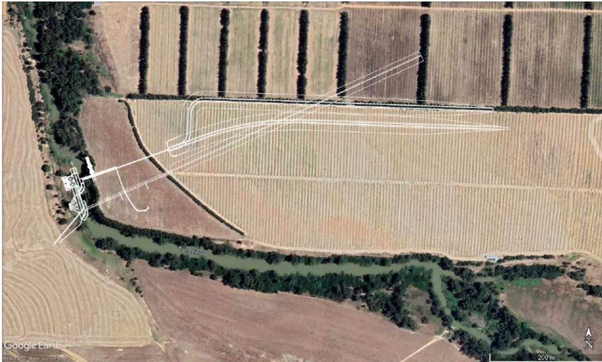
Figure 2: View of the Initial and Final Positions of the BRVAS Weir and Abstraction Works with Alternative Positions for the Earth-fill Embankment
