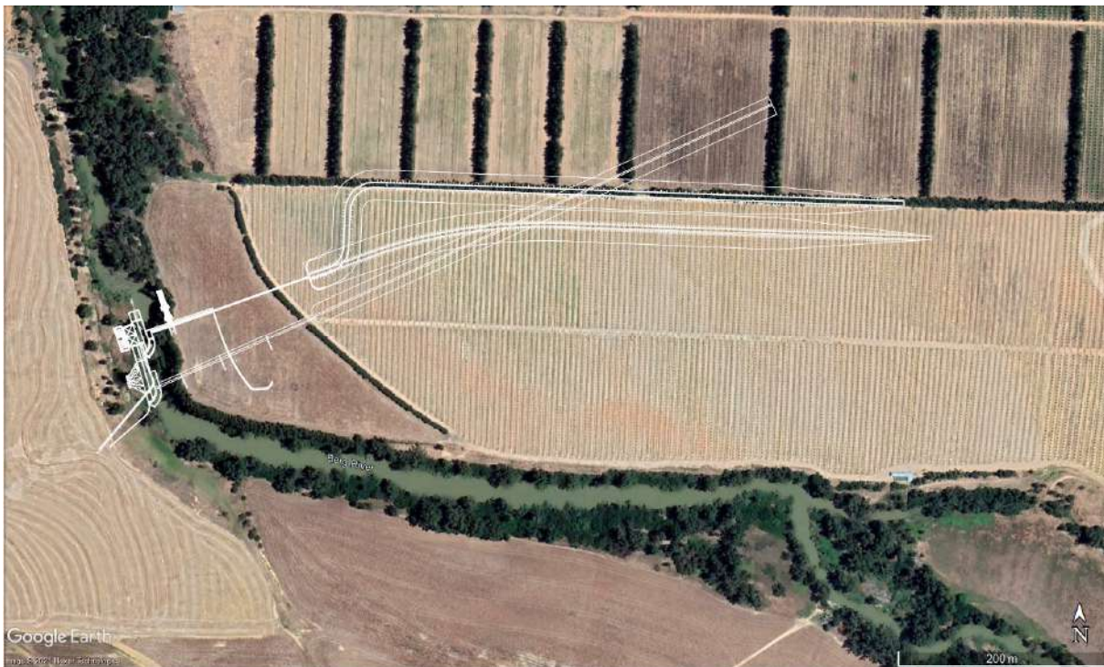
Figure 7: Alternative Positions for the Earth-fill Embankment
