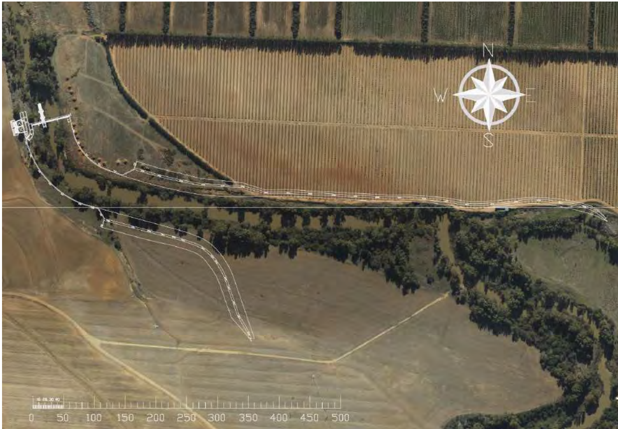
Figure 9-11: Option C plan layout of the weir, abstraction works and berms/walls
