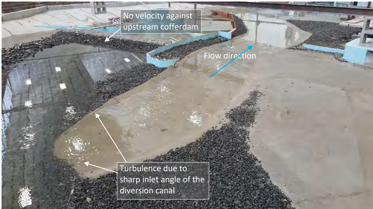
Figure 10-11: Temporary works layout of Option C for a 2-year ARI-flood (183 m 3 /s), downstream view from right bank floodplain
