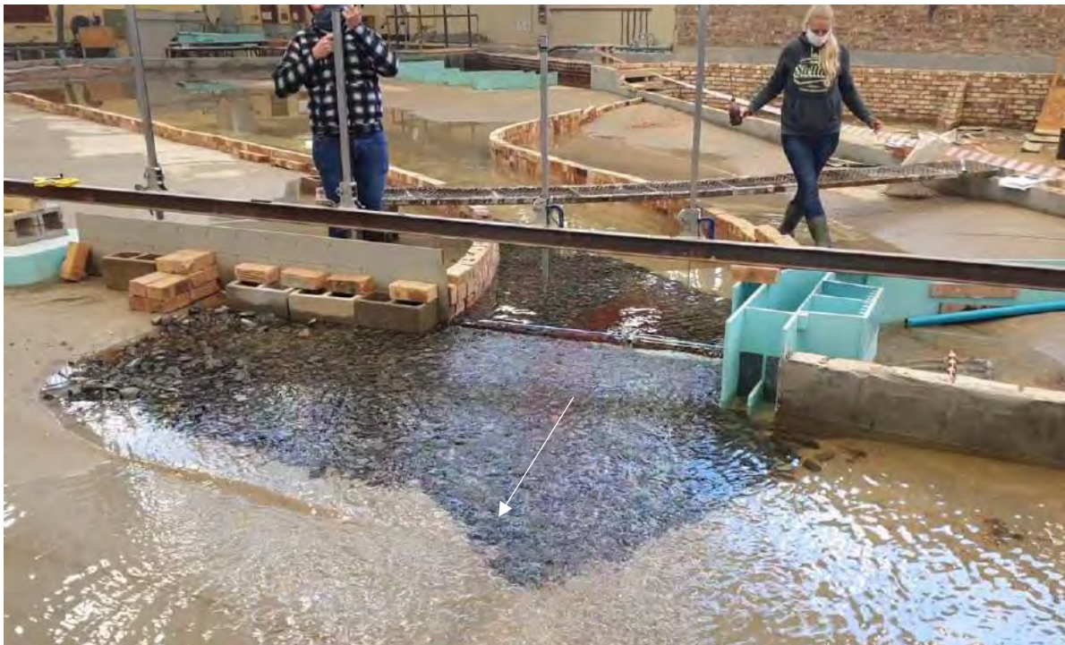
Figure 9-12: Option A model study test to optimize the berm locations at Q_{2cc} ( 210 \text{ m}^3/\text{s} ) and a weir length of 60 m viewed from downstream
