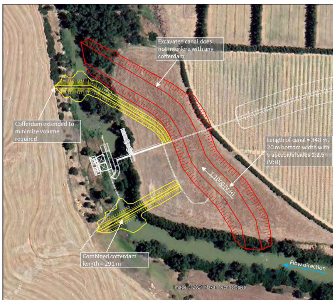
Figure 10-5: Option C, cofferdam and diversion canal footprint
