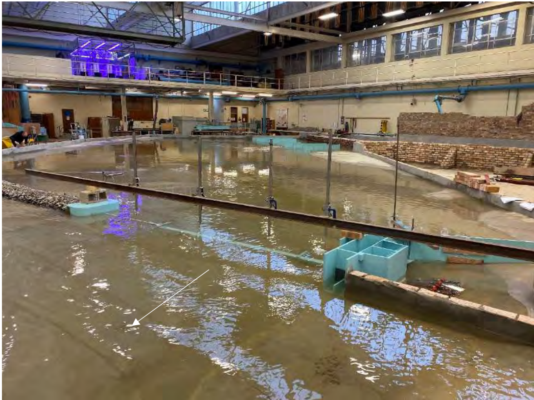
Figure 9-8: Weir with 4 notches, abstraction works and berm during the RMF (4 494 m 3 /s) as viewed from downstream
