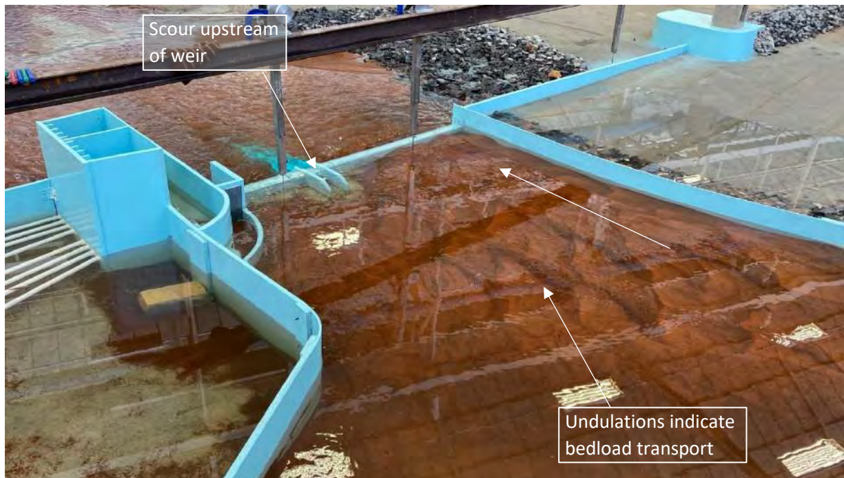
Figure 9-27: Upstream sediment transport at Q_{2cc} ( 210 \text{ m}^3/\text{s} ) and significant scour upstream, against the weir
