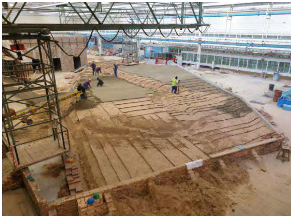
Figure 6-2: Construction of the physical model topography of the Berg River and its floodplains
