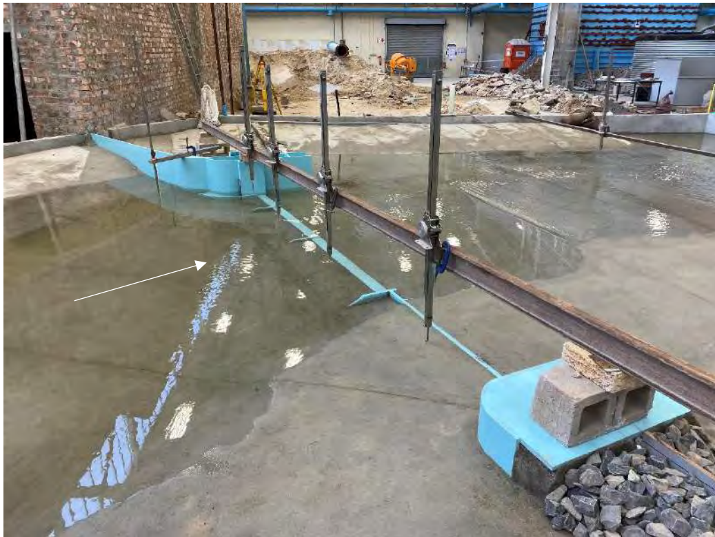
Figure 9-5: 1:40 scale model weir with 4 notches, abstraction works and berm during the Q5cc flood (424 m 3 /s) as viewed from the right bank side
