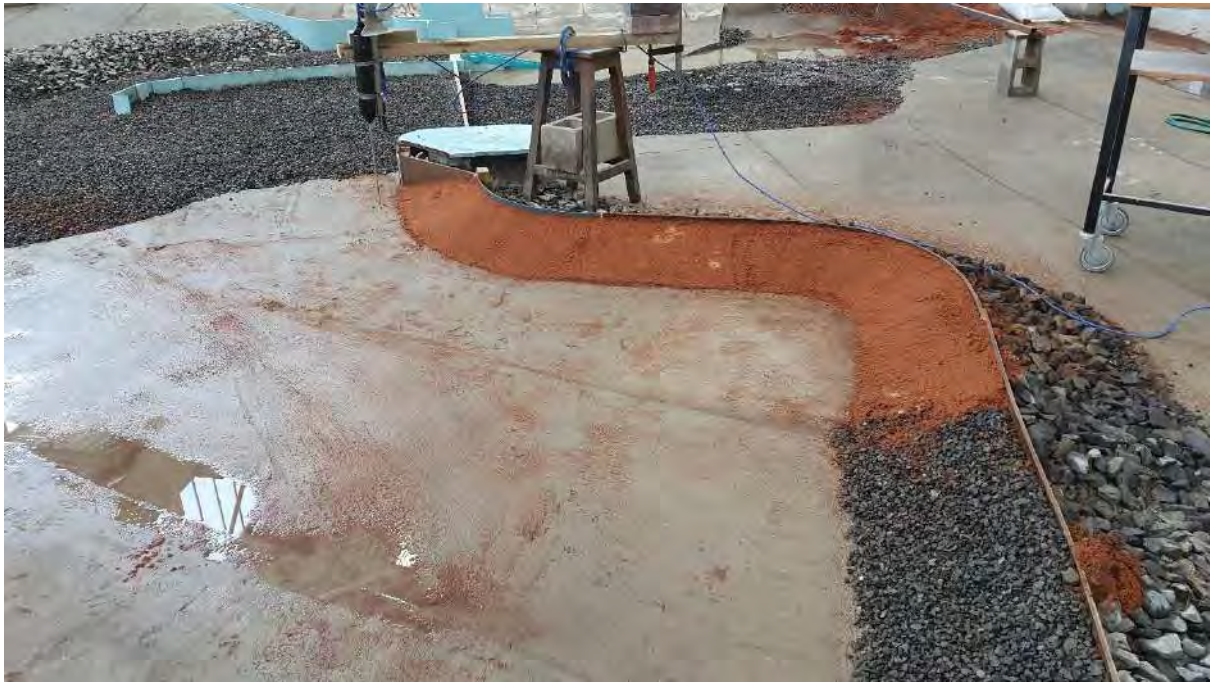
Figure 9-41: Movable bed setup of the s-berm test for erosion protection
