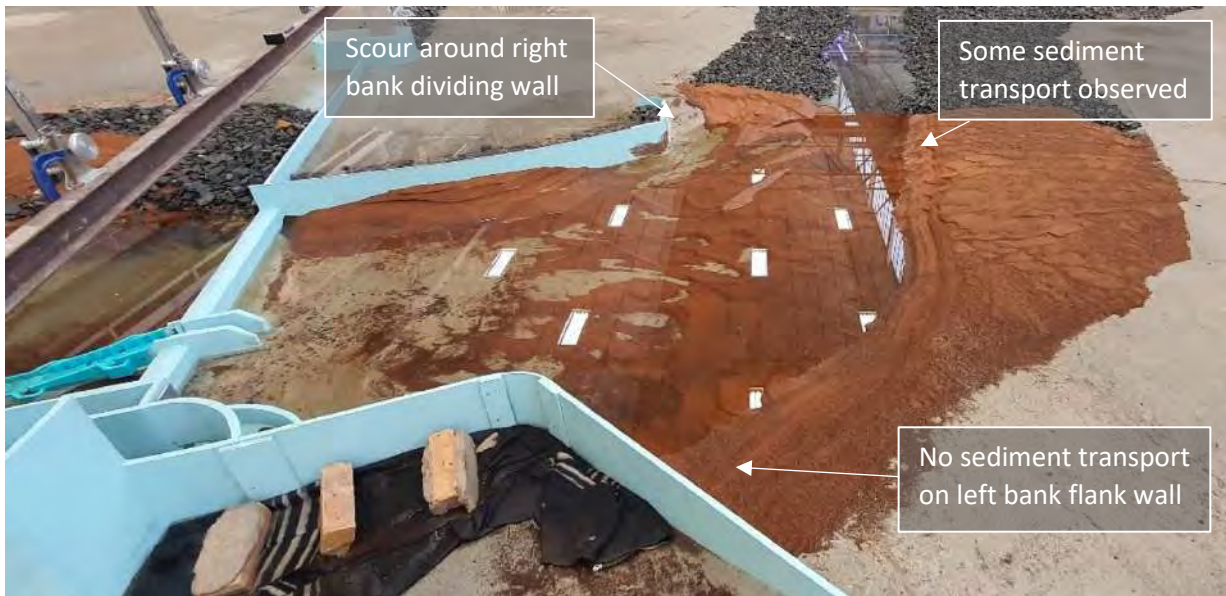
Figure 9-33: Upstream view of riverbed after Q50cc (1169 m 3 /s) showing areas of deposition, scour and no sediment transport
