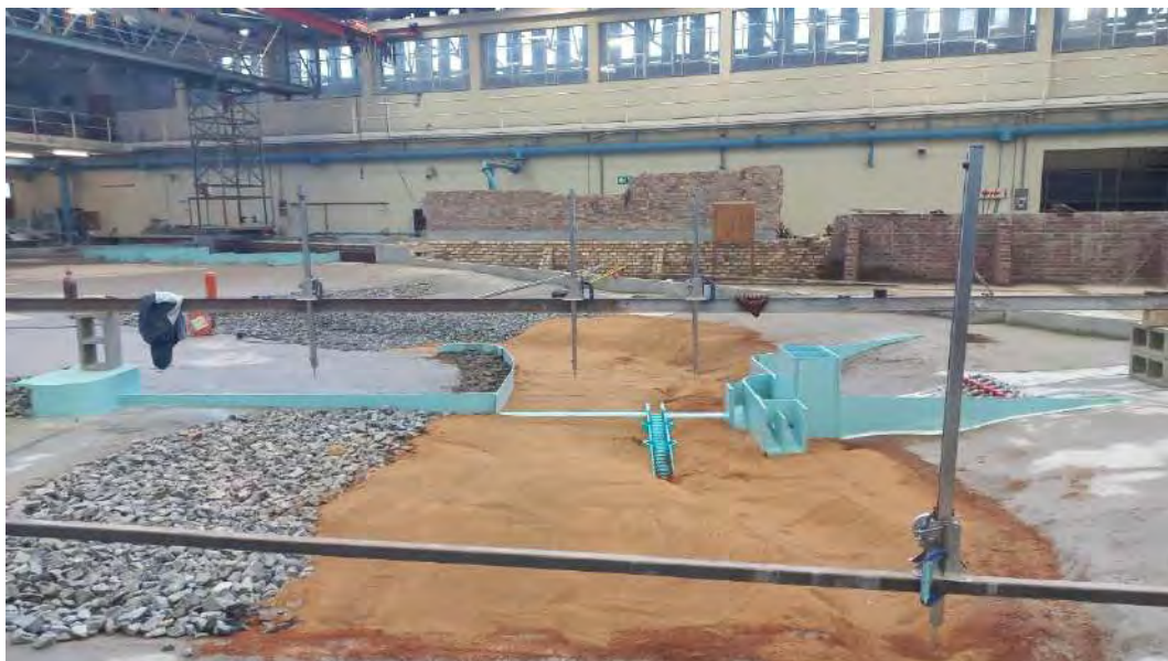
Figure 6-6: Movable bed tests of the final abstraction works design viewed from downstream
