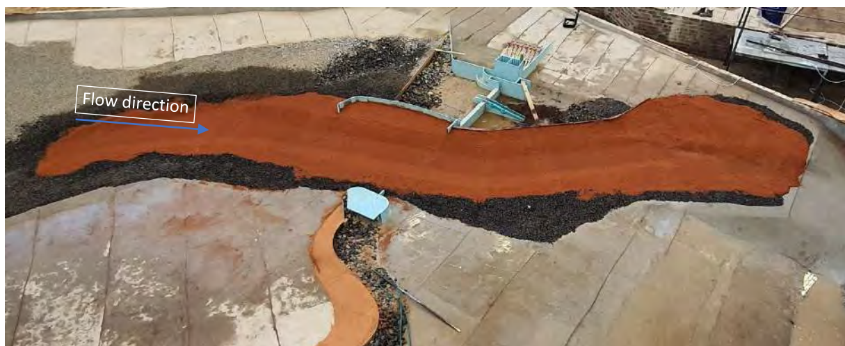
Figure 10-17: Movable bed setup for the modified option C layout
