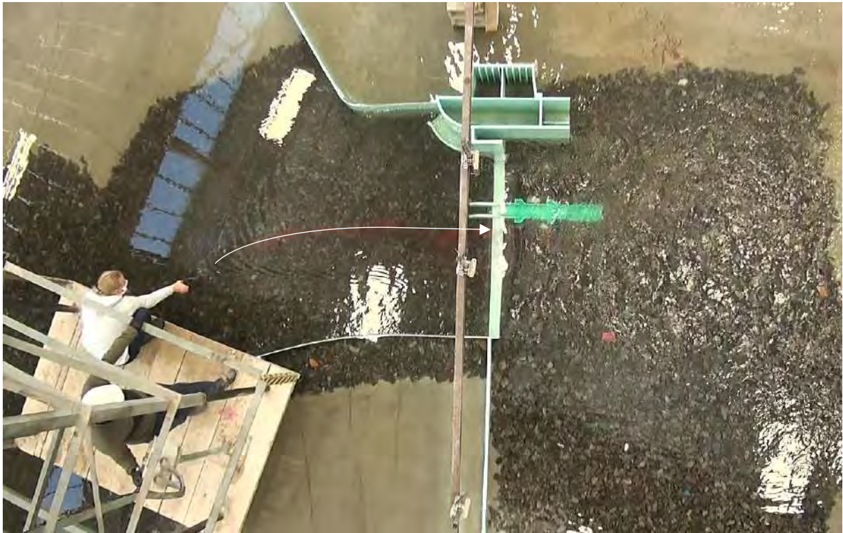
Figure 9-20: Flow is guided by the right bank guide wall and flows over the weir perpendicular to the weir Q50cc
