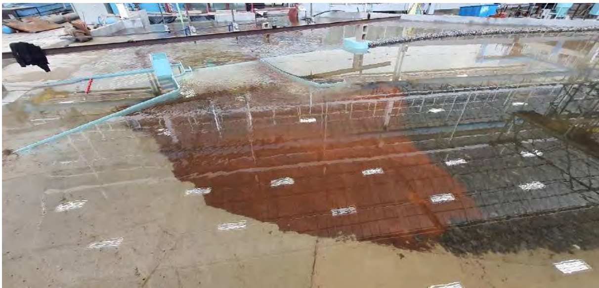
Figure 9-34: Downstream view of Q100cc (1468 m 3 /s), left bank flank wall with abstraction works visible just above water surface, right bank is spilling over the 100 m broad crest weir
