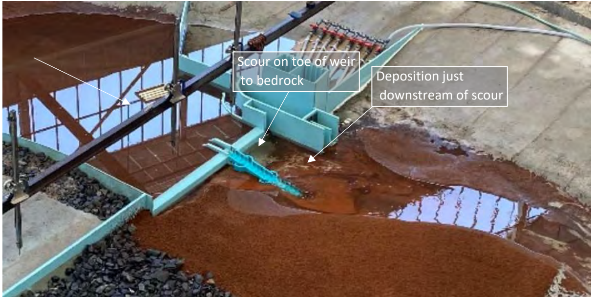
Figure 9-25: At low flow the toe of the weir is scoured to bedrock with deposition just downstream of the scour hole formed ( Q = 10 \text{ m}^3/\text{s} )
