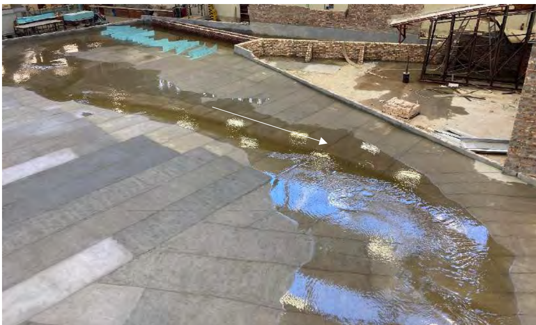
Figure 9-2: Photograph of the physical model of the natural BRVAS for the Q10cc (613 m 3 /s)
