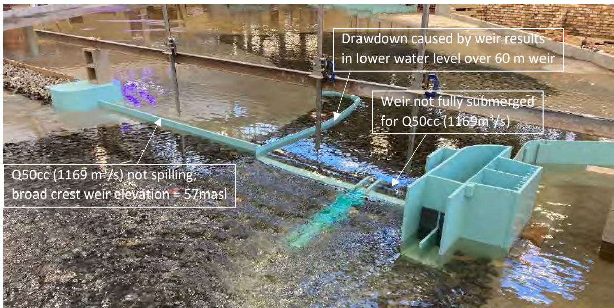
Figure 9-21: The 100 m broad crest weir and guide wall is not spilling for the Q50cc (1169 m 3 /s) flood peak
