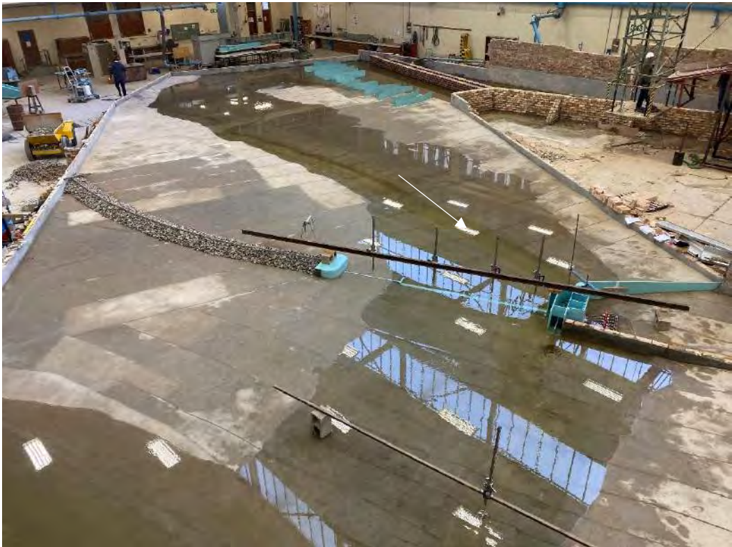
Figure 9-6: Weir with 4 notches, abstraction works and berm during the Q5cc flood (424 m 3 /s) as viewed from downstream
