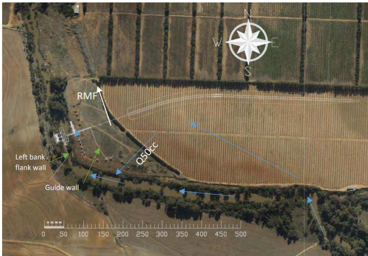
Figure 9-16: Option B2 plan layout of the weir, abstraction works, berm and proposed dividing wall (right bank) and flank wall (left bank)
