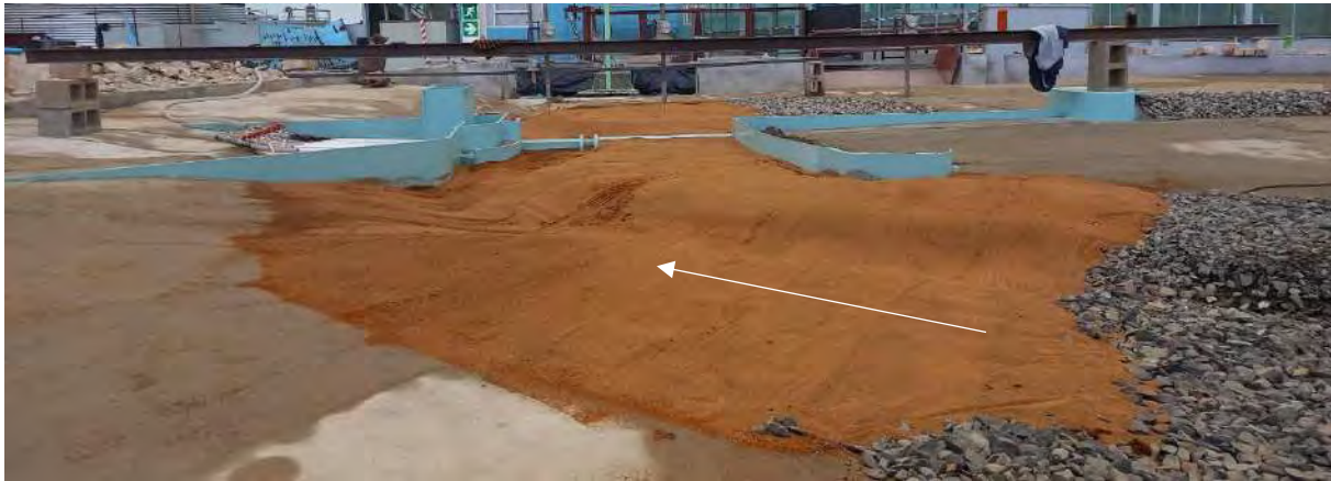
Figure 9-24: Movable bed setup with sediment shaped to the 2021 survey of the river
