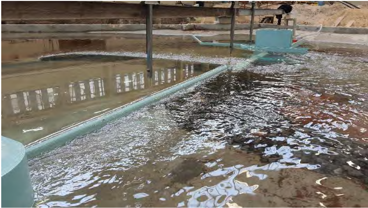
Figure 9-35: Upstream view of Q100cc (1468 m 3 /s) flowing over partially submerged 60 m Crump weir
