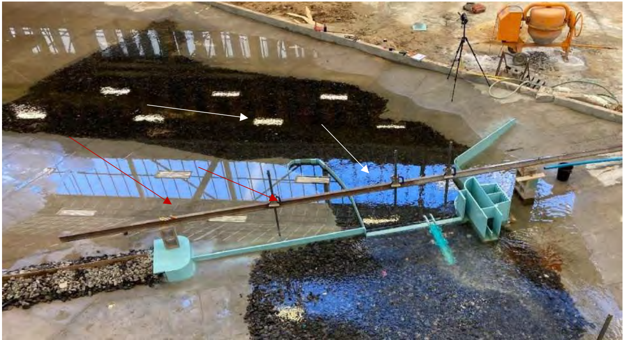
Figure 9-22: Q5cc (424 m 3 /s) guide wall is required to prevent flow from flowing over floodplain (red arrows), bypassing the abstraction works, guide wall redirects flow (white arrows) and aligns the flow with the abstraction works and weir
