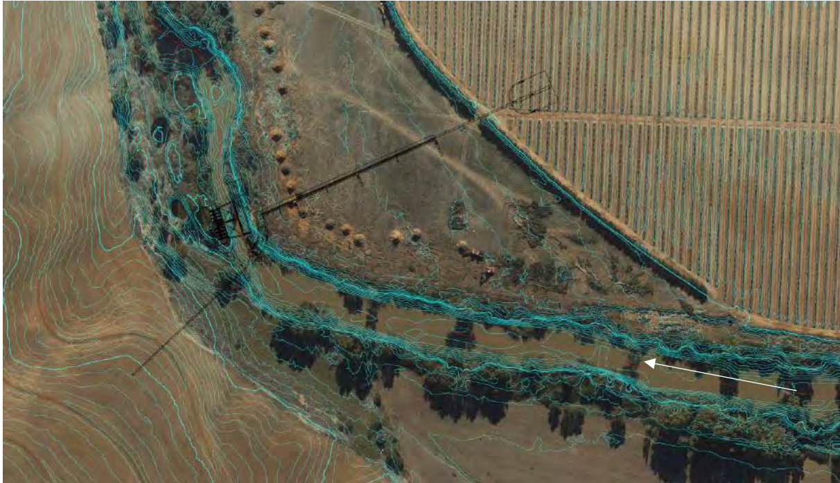
Figure 9-3: Plan layout of the proposed BRVAS abstraction works and weir shown on the 2021 topographical survey and based on the 2012 feasibility study design concept
