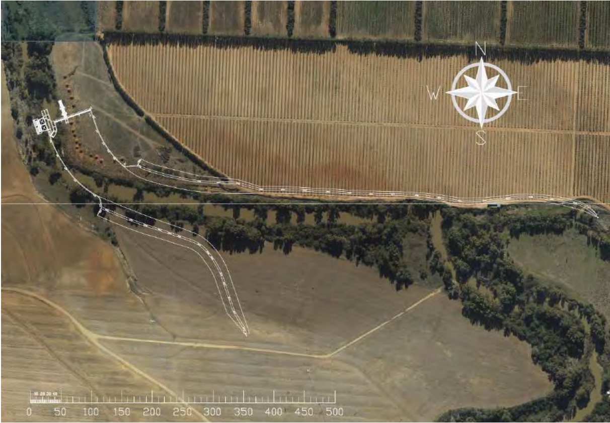
Figure 9-10: Option B plan layout of the weir, abstraction works and berms/walls
