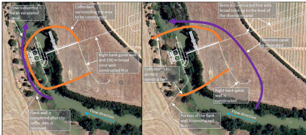
Figure 10-2: Temporary works layout for Option B (left) and Option C (right)
