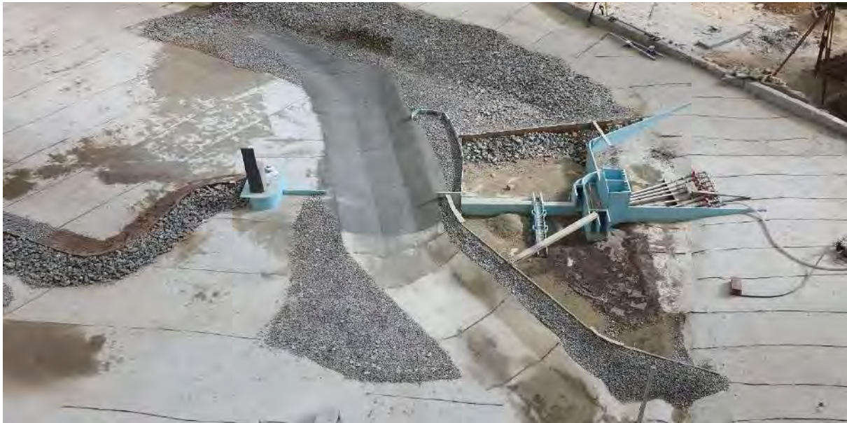
Figure 10-14: Modified option C layout constructed as a fixed bed model viewed from downstream
