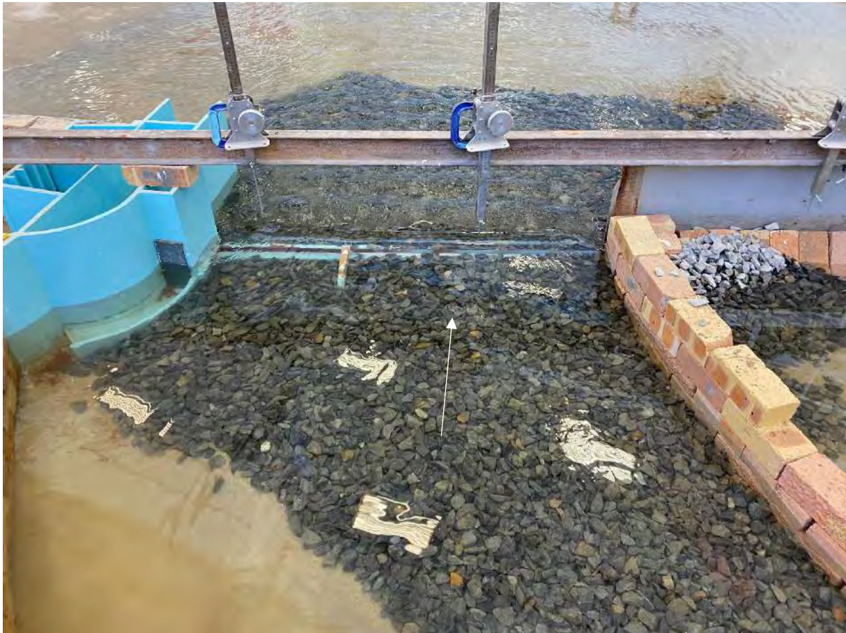
Figure 9-14: Photograph of option A physical model study with improved flow patterns for the new weir and berm layout during the Q10cc (613 m 3 /s) viewed from upstream
