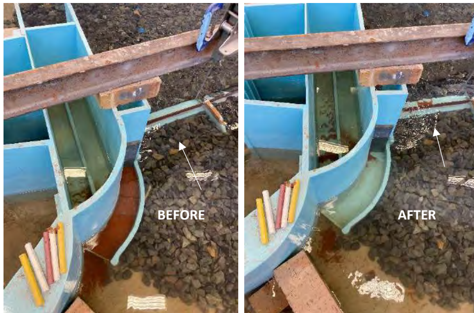
Figure 9-15: Option A model study test showing the self-scour abilities of the improved berm and weir design (without opening the boulder gate) during the Q10cc flood (613 m 3 /s) viewed from upstream
