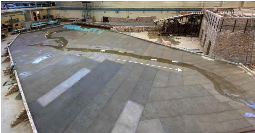
Figure 9-1: Photograph of the physical model of the natural BRVAS site for the Q2cc (210 m 3 /s)
