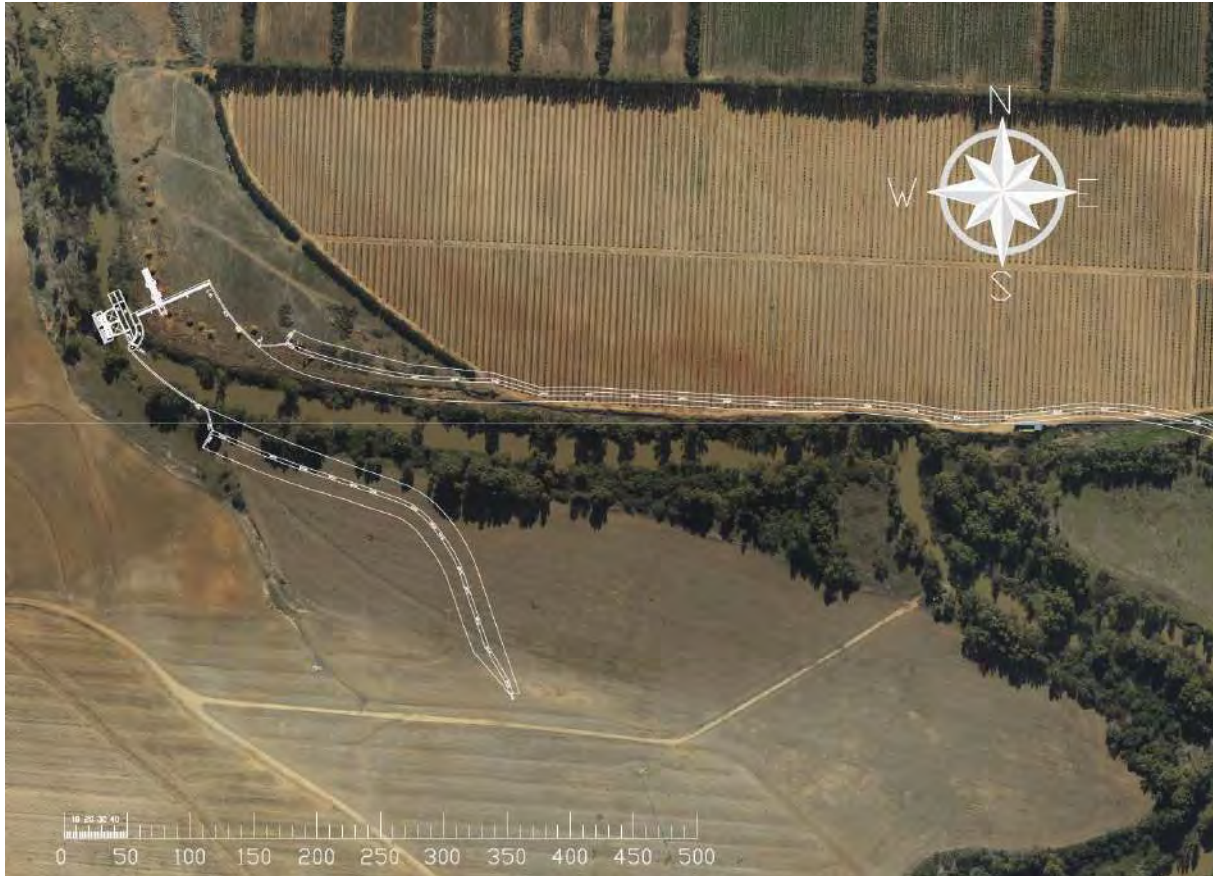
Figure 9-9: Option A plan layout of the weir, abstraction works and berms/walls
