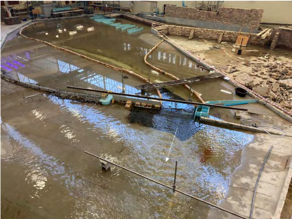
Figure 9-13: Photograph of option A physical model study showing optimized berm locations and weir design for the Q50cc (1 169 m 3 /s) viewed from downstream
