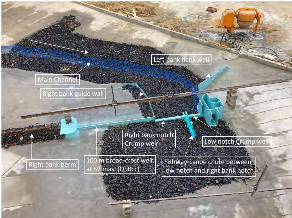
Figure 9-18: Fixed bed tests, Option B2, gravel used to obtain surveyed bed level before the movable bed sediment is introduced into the model
