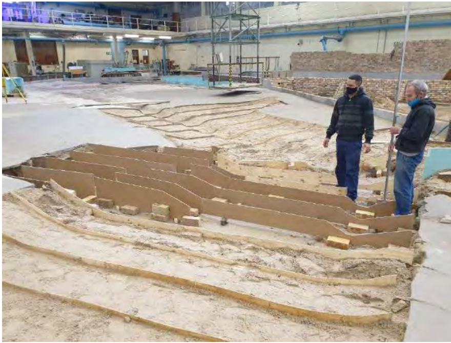
Figure 6-3: Modification of the physical model topography by incorporating new templates that are representative of the new 2021 surveyed levels
