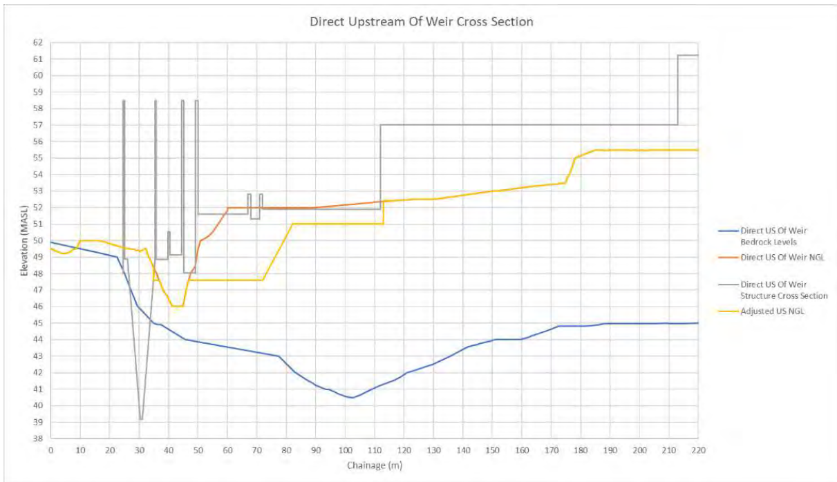
Figure A1-3: Proposed BRVAS weir sections at the weir viewed looking downstream
