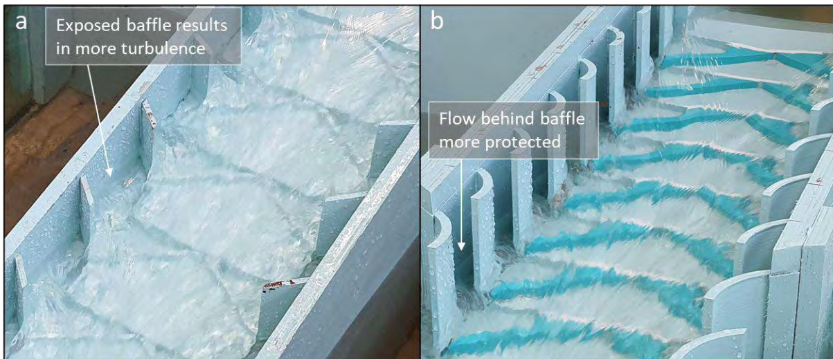
Figure 11-16: Comparison of turbulence between angled baffles and 1m radius baffles
