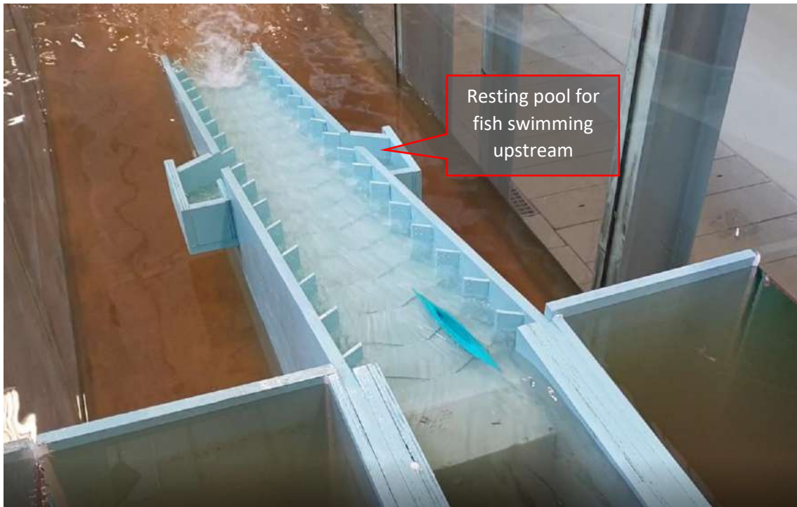
Figure 11-3: Fishway-canoe chute model at a discharge of about 8 m 3 /s in the chute (H = 1.2m) viewed from upstream
