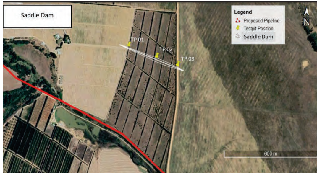
Figure 8: Saddle Dam Testpit Positions
