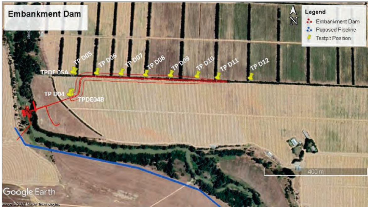
Figure 7: Embankment Testpit Positions
