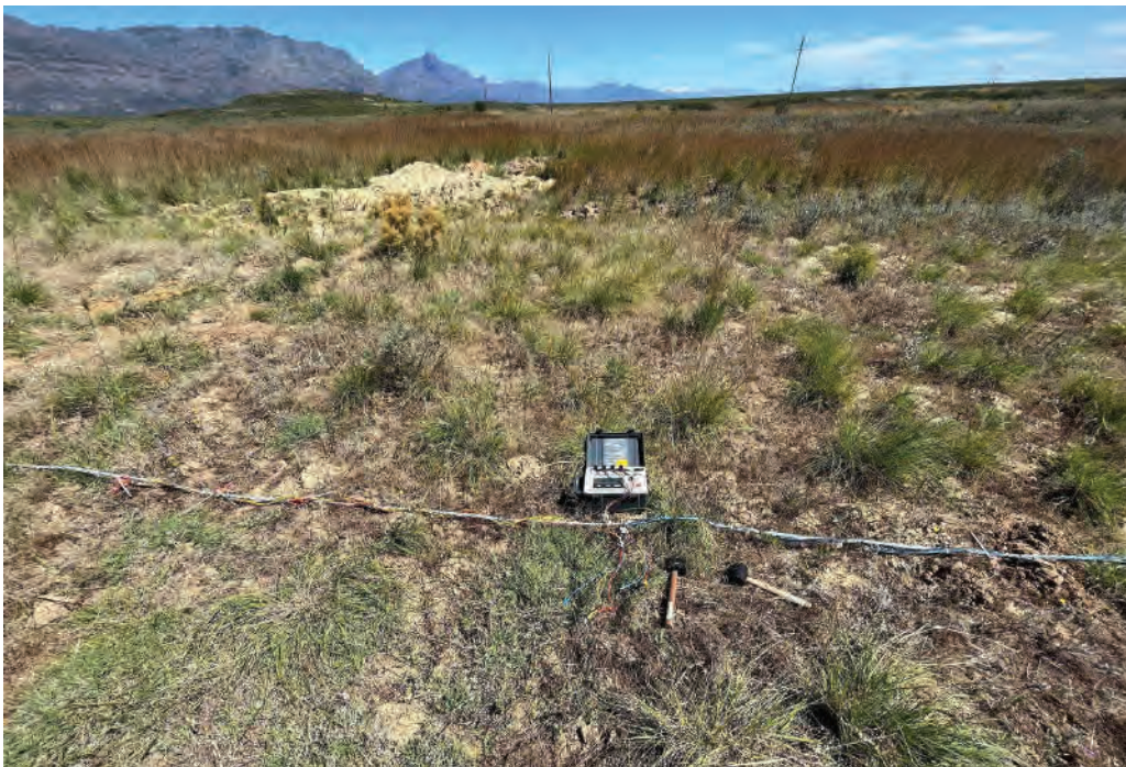
FIGURE 3: SOIL RESISTIVITY MEASUREMENT ILLUSTRATION
